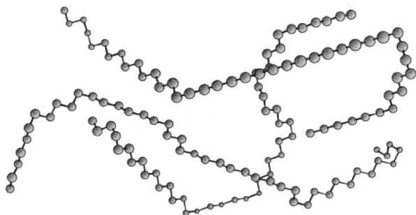
Figure 3. Schematic structure model for the noncrystalline sPP chains just after quenched at 0 °C from the melt.
